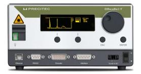
The latest generation of the proven CHRocodile sensor line offers an unrivaled speed of 70,000 measurements / second. The CHRocodile 2 IT optical sensor works with infrared light and is perfectly suited for distance and non-contact thickness measurement of non-transparent materials from one side.
