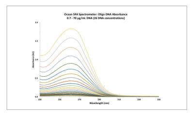
Even a small amount of protein contamination in DNA solution can have a large effect on UV absorbance. In this case, SR4 demonstrated good linearity up to 2 AU.
