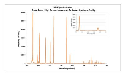
The HR6 provides broadband, high resolution performance for emission and other measurements.
