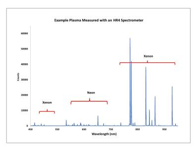
As a high-resolution, thermally stable spectrometer, the HR4 is ideal for monitoring the emission peaks of gases used in semiconductor and other manufacturing processes.
